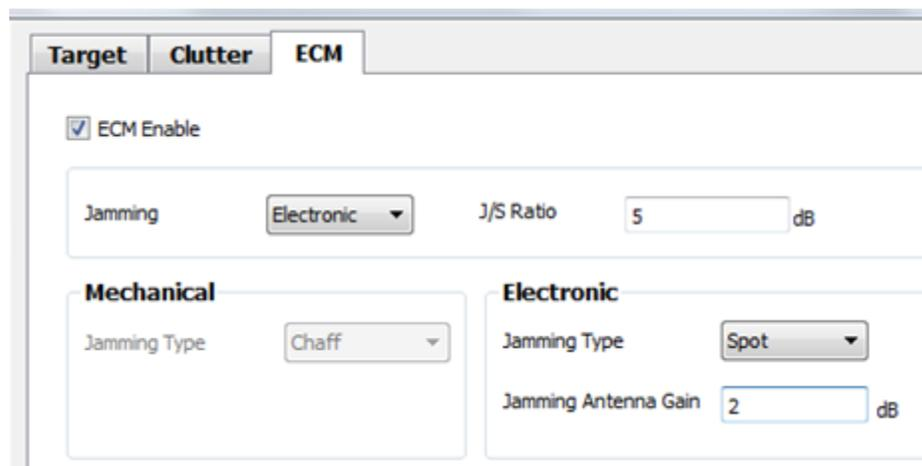
Figure. UTS-RTS Target On-board jammer modeling features
